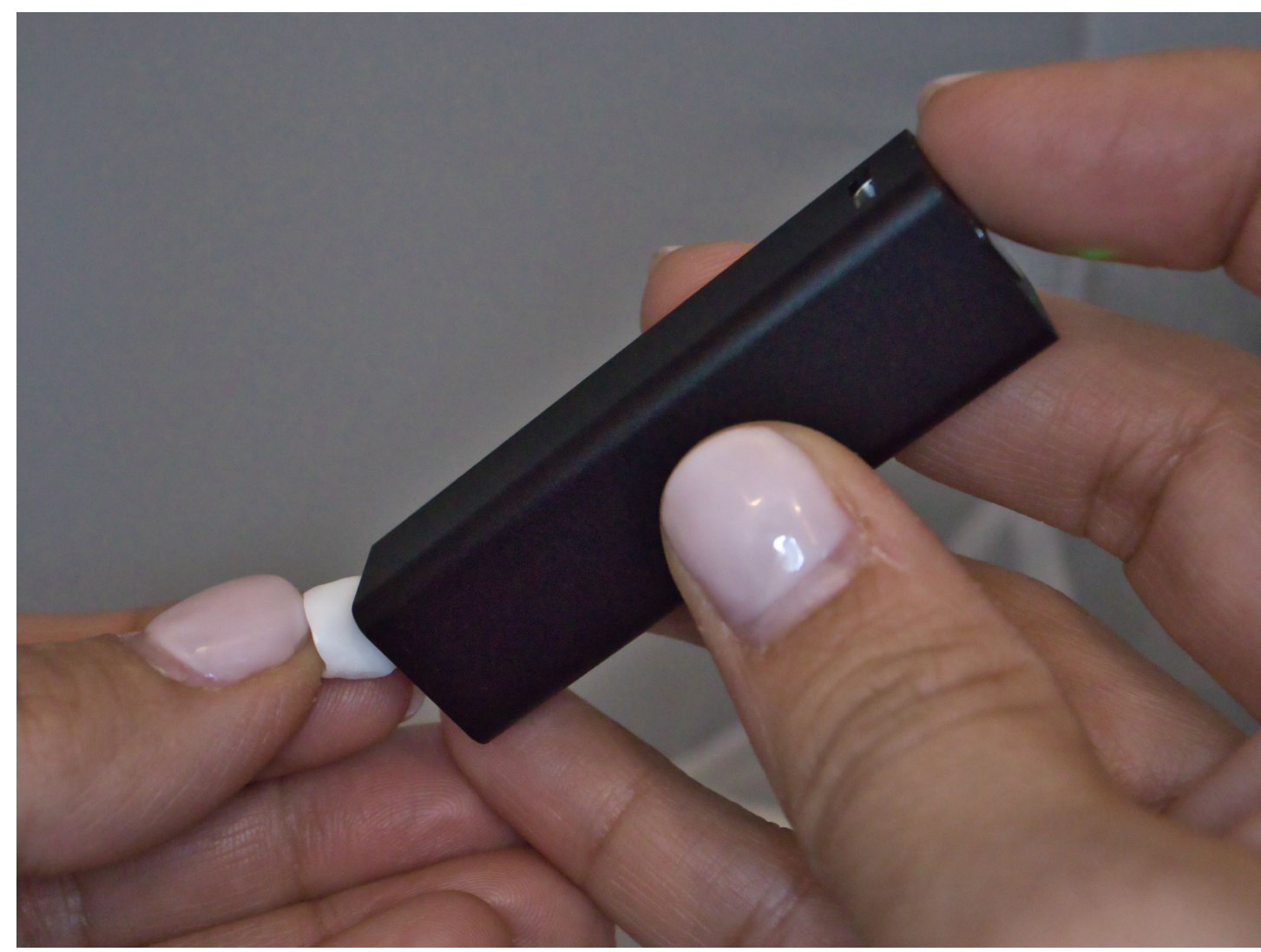
Figure 9. Wireless Bluetooth sensor connected to SmileShade software contacts surface of the crown and veneer.
